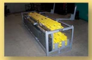
Unique rack (storage) system can be lifted on all sides with a fork lift or from above via lifting eyes.
